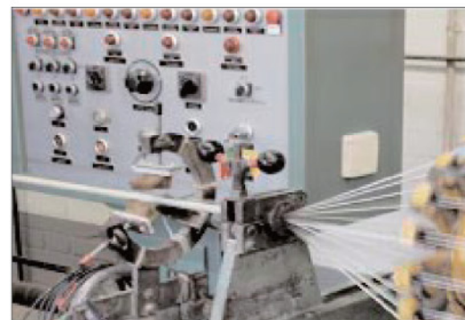
Stranding of conductors
